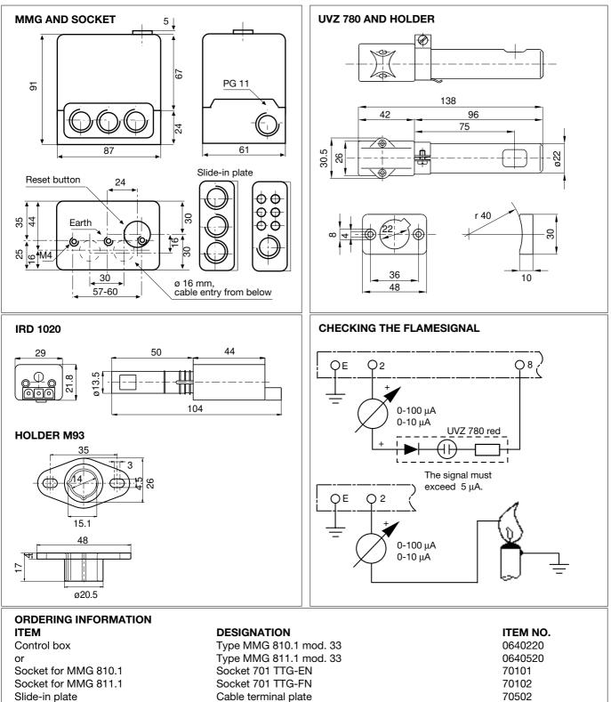
Slide-in plate or Flame detector Flame detector Flame detector IRD mounting flange UVZ mounting flange Flame detector cable Type MMG 810.1 mod. 33 Type MMG 811.1 mod. 33 Socket 701 TTG-EN Socket 701 TTG-FN Cable terminal plate PG-plate IRD 1020 end-on viewing IRD 1020 side-on left IRD 1020 side-on right UVZ 780 red IRD Holder M93 UVZ Holder 3-wire, 0.6 m
