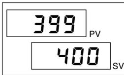
PV Displays the value of the Process Variable.
