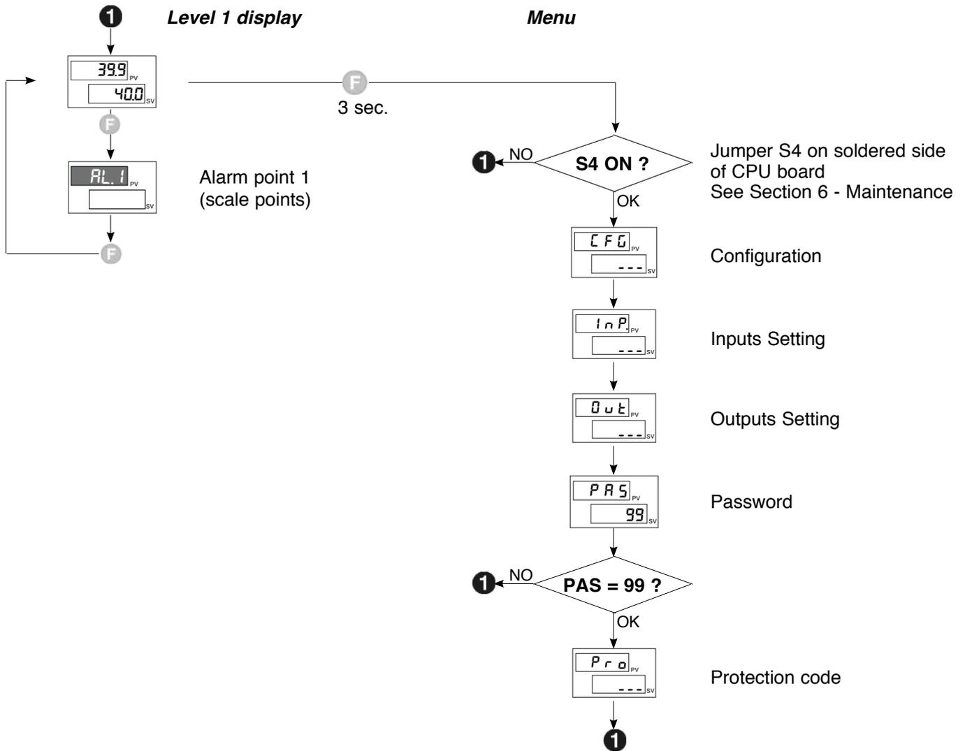
This menu is used to configurare the control parameters in the Easy mode.
