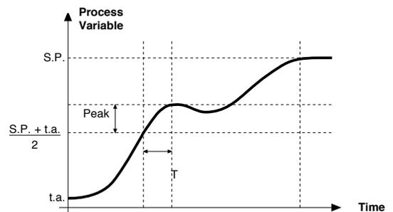
The procedure runs automatically until finished, when the new PID parameters are stored: proportional band, integral and derivative times calculated for the active action (heating or cooling). In case of double action (heating or cooling), parameters for the opposite action are calculated by maintaining the initial ratio between parameters (ex.:  $CPb = HPb * K$ ; where  $K = CPb / HPb$  when self-tuning starts). When finished, the **Stu** code is automatically cancelled.
