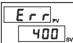
*Err* third wire broken for PT100, PTC or input values lower than minimum limits (e.g. for TC with wrong connection)
