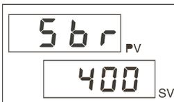
*5br* broken probe or input values higher than maximum limits
