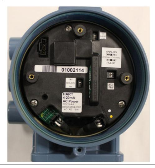
Figure 6-1: Electronics Stack and Hardware Switches
