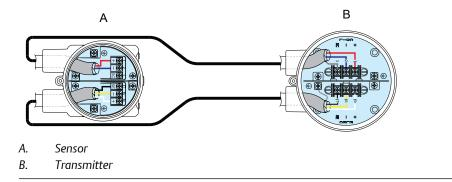
Figure 4-12: Remote junction box views (wall mount)
