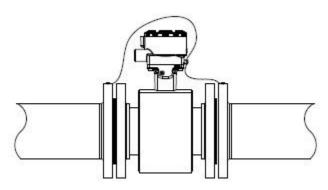
Figure 3-8: Grounding with grounding rings or lining protectors in conductive pipe
