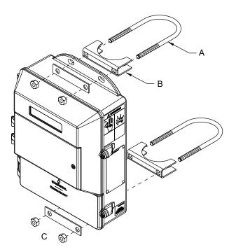
Figure 4-4: Wall mount transmitter mounting hardware
