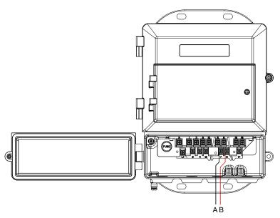
Figure 4-20: Analog output wiring, internal power (wall mount)
