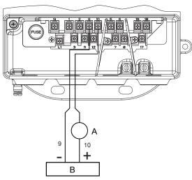
Figure 6-14: Connect discrete output to relay or control system input (wall mount)
