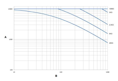
Figure 6-3: Output Option Code A—Maximum Frequency vs. Cable Length
