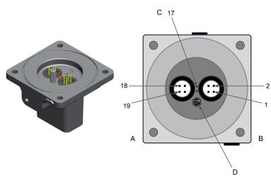
Figure 12-2: Sensor Adapter Feed-through Pins
