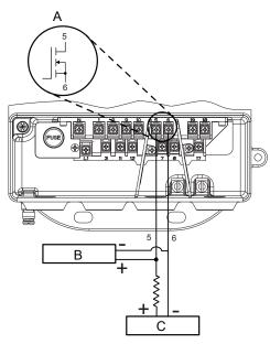
Figure 6-10: Connecting to an electronic totalizer/counter with external power supply (wall mount)
