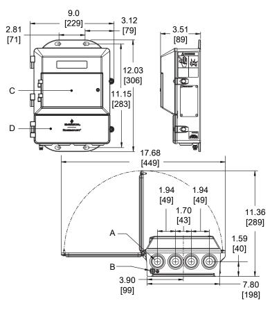
Figure 4-2: Wall mount transmitter dimensional drawing
