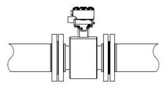
Figure 3-11: Grounding for line sizes 10-in. and larger
