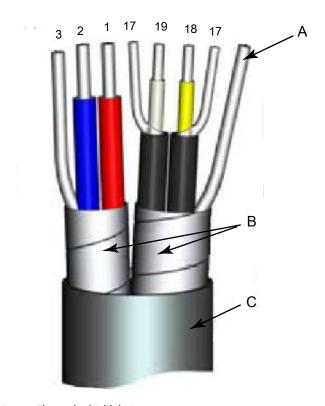
Figure 4-9: Combination coil and electrode cable
