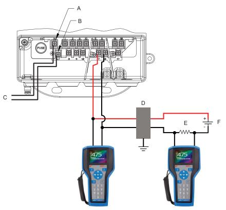
Figure C-8: Wiring diagram—Field Communicator with transmitter external analog power
