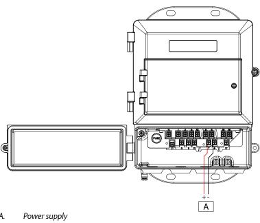
Figure 4-22: Analog output wiring, external power (wall mount)
