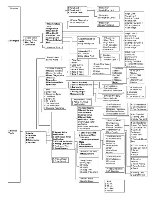
Figure 7-9: Field Communicator Dashboard Menu Tree (HART v7.1, part 2)
