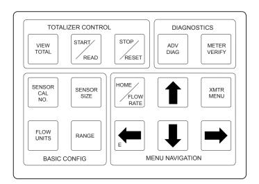
Figure 7-2: Local Operator Interface and Character Display
