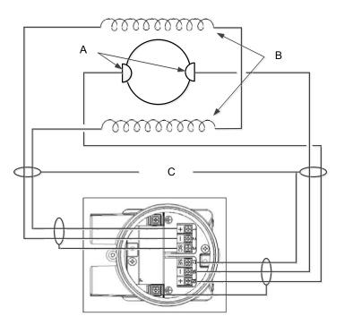
Figure 12-1: Sensor Circuit Diagram (Simplified)
