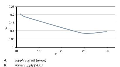
Figure 4-18: Low power DC current requirements
