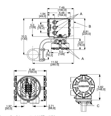
Figure 4-1: Field mount transmitter dimensional drawing
