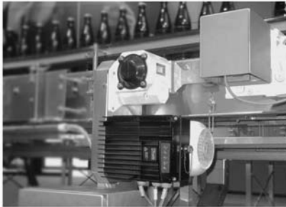
Figure 1.11: FCD 300 on bottling conveyor
