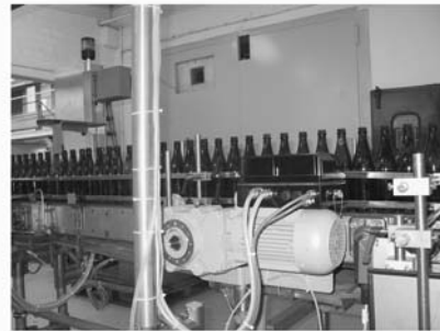
Figure 1.12: FCD 300 on bottling conveyor
