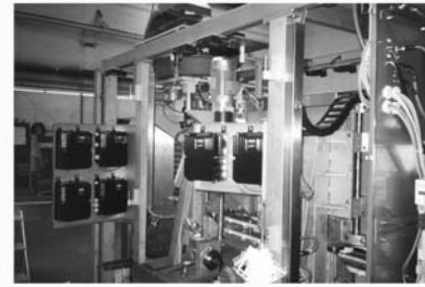
Figure 1.13: Decentral motor controls integrated in packaging machine
