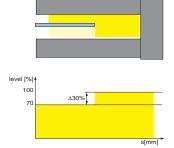
Reliable edge detection at max. 70 % transparency of the material webs
