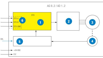
Simplified block diagram of the BLDC drive: 1 Impulse block / 2 Power stage / 3 Motor / 4 Multiturn encoder / 5 Drive control / 6 Galvanic isolation
