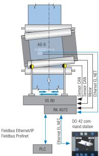
Web guiding system with sensor positioning and interface module
