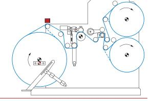
ELWINDER WSB91 on slitter rewinder
