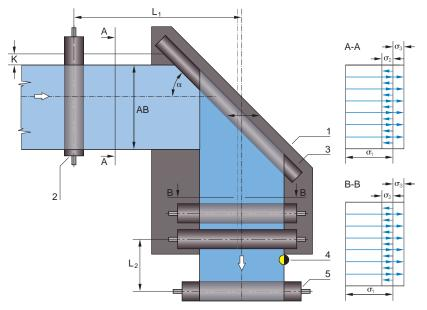
A-A Web tension distribution at infeed Web tension distribution at exit
