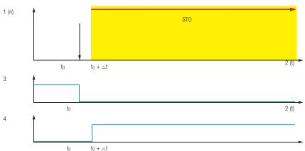
Prevention of starting by means of the activation of the STO safety function: 1 Speed (n) / 2 Time (t) / 3 Request (STO input) / 4 Status
