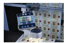
Color line sensor FE 52 on roller inspection machine
