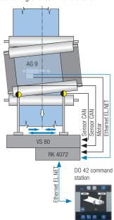
Web guiding system with sensor positioning and standard interface
