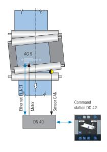
Web guiding system with standard interface Ethernet/IP/Profinet
