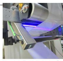
Web center detection of film with blue light wide band sensor FR 65
