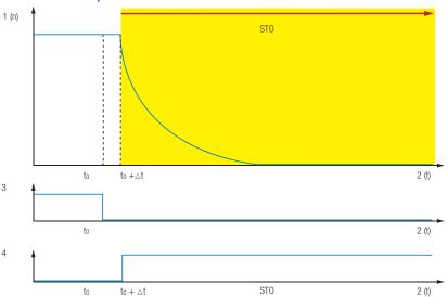
Prevention of starting by means of the activation of the STO safety function: 1 Speed (n) / 2 Time (t) / 3 Request (STO input) / 4 Status
