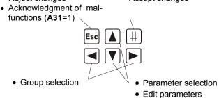
To program, press the # key (Enter). The menu consists of several groups which are identified with the letters A, B, C and so on. Select the groups with the arrow keys (i.e., \ and ). Press the # key again to access the parameters of the selected group.
