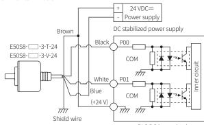
PLC DC input circuit
